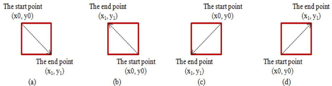
Figure 3. Models of cropping area (a) the top left to the bottom right, (b) the right down to the top left, (c) top right to the bottom left, (d) the bottom left to the top right
